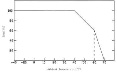
If being used in higher ambient temperatures, ensure the load on the LED driver is de-rated in accordance with this chart. Failure to do so could lead to a failure, which is not covered by the warranty
